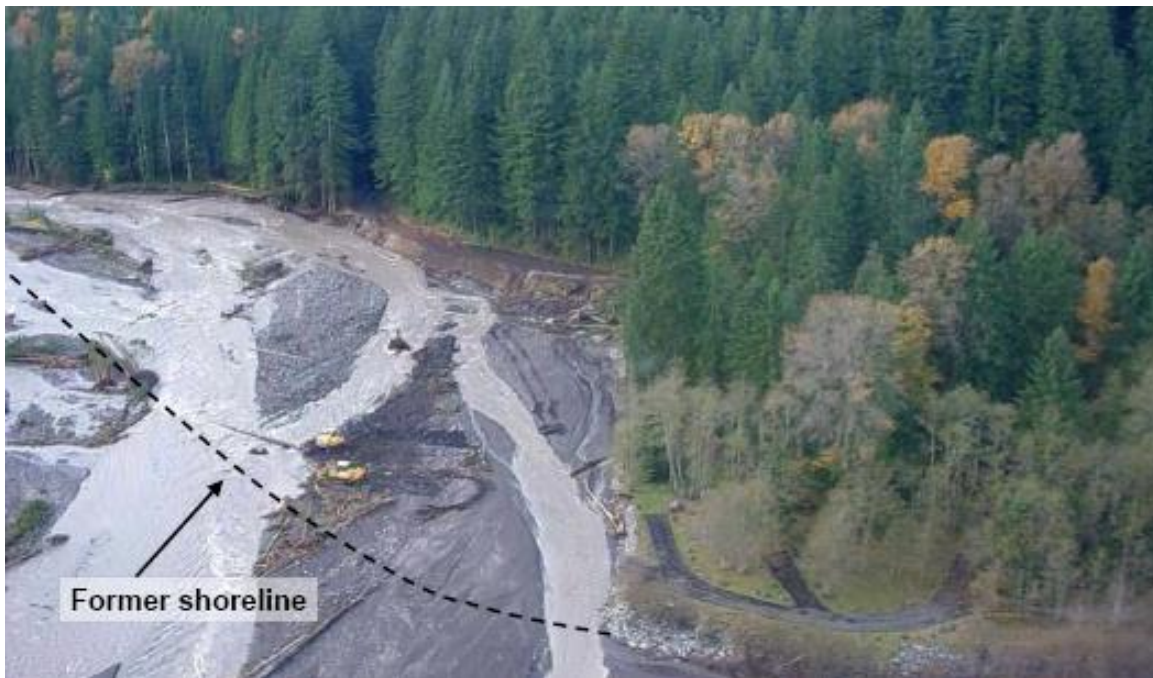
Figure 6.96. Aerial View of Sunshine Point Damage Area along the Upper Nisqually River after November 2006 Flood Event and Repair of Revetment and Levee
